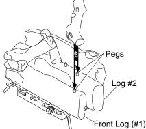
Figure 33 - Installing Crossover Log (#6) (CCL3930NTA Shown)
